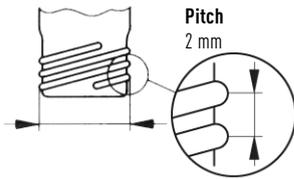
**GL 14** – outer- $\varnothing$  = 14 mm
