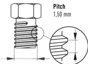
**M 12** – outer- $\varnothing$  = 12 mm
