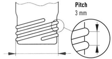
**GL 25** – outer- $\varnothing$  = 25 mm
