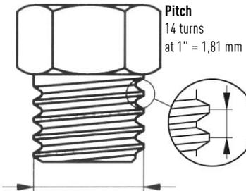
**G 5/8"** – outer- $\varnothing$  = 22,8 mm
