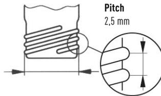
**GL 18** – outer- $\varnothing$  = 18 mm
