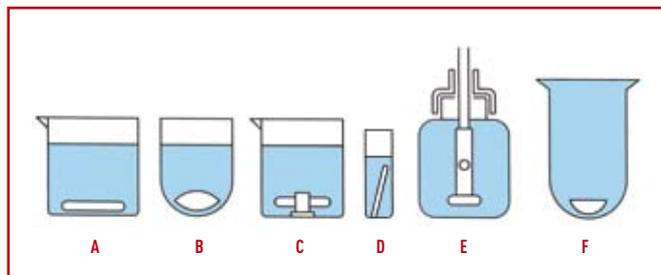
A Cylindrical magnetic stirring bar » B Oval or Egg-shaped magnetic stirring bar » C Magnetic stirring bar with bearing neck » D Magnetic stirring bar for cuvettes » E Magnetic stirring bar for culture bottles » F Custom manufacture for flanged reactors
