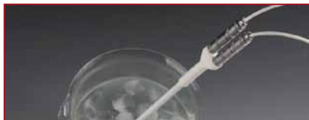
Field-proven method of determination: Put the temperature probe in an ice cold water bath and let it reach a steady-state. Then transfer it quickly to a column of steam and monitor its resistance until a steady state is reached again.
