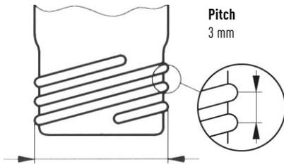
**GL 32** – outer- $\varnothing$  = 32 mm
