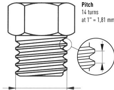
**G 3/4"** – outer- $\varnothing$  = 26,3 mm
