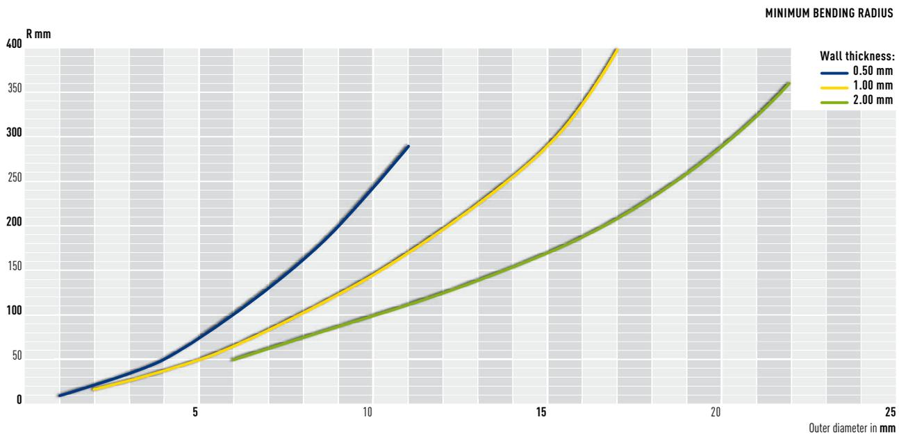
**Example:** A PTFE tubing with outer diameter 10 mm and a wall thickness of 2 mm has a minimum bending radius of 100 mm.
