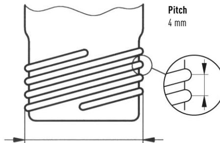
**GL 45** – outer- $\varnothing$  = 45 mm
