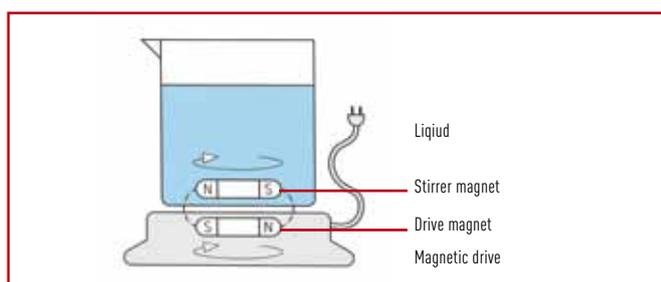
The **stirrer magnet** is a bar magnet encapsulated in a material which protects the magnet and prevents contamination of the liquid medium.
