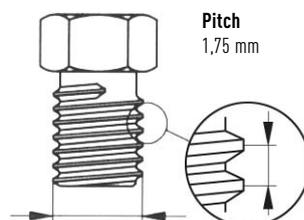
**M 16** – outer- $\varnothing$  = 16 mm
