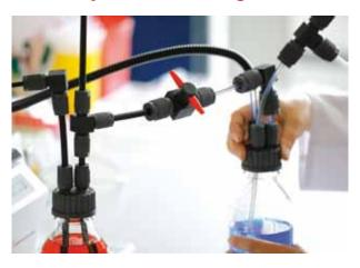
By adding conductive particles, these components become electroconductive and can be used for explosive applications.
